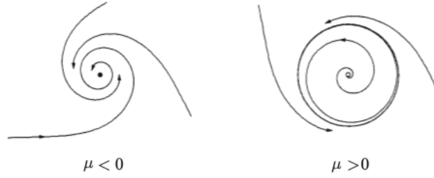
Figure 10 Canonical phase portraits of the supercritical Hopf bifurcation in (54): \mu < 0 on the left and \mu > 0 on the right.
